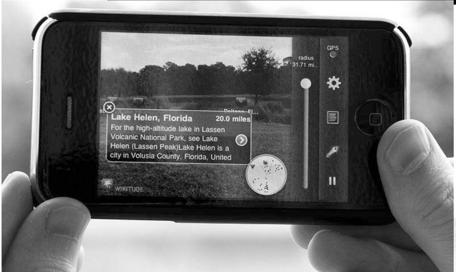
Wikitude World Browser on the iPhone 3GS uses GPS and a solid state compass
